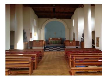
The builder was Mr William Darby of Knebworth. The special bricks and pantiles were made in his brickyard at Rabley Heath. Local builders were responsible for cutting the great 12" x 18" tie beams of the roof from the round and for cutting and fitting all the woodwork in the church including the panels of the roof, the ambos, choir stalls and the altar.
